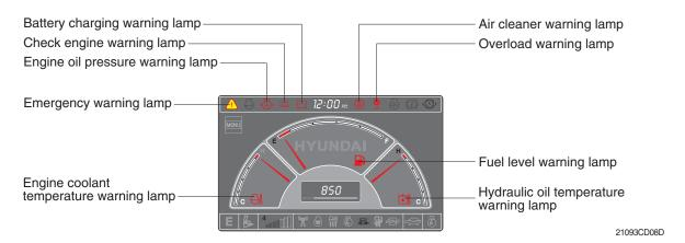
Each warning lamp on the top of the LCD pops up on the center of LCD and the buzzer sounds
